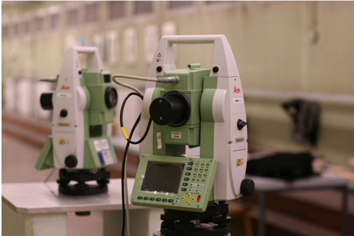
Figure 8. Image assisted total stations with frame sensor in the focal plane of the telescope.
