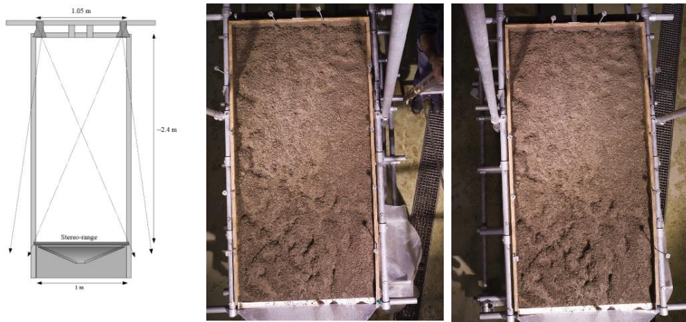
Figure 2. Setup with two camera stations above the soil surface (left) Stereo image pair of the flume surface.
